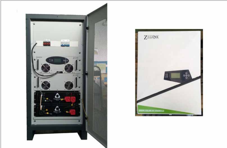
Figure 8: Converter for homes and streetlighting (left), inverter for non-residential buildings (right) (Source: ZIGOR Research & Development A.I.E).
