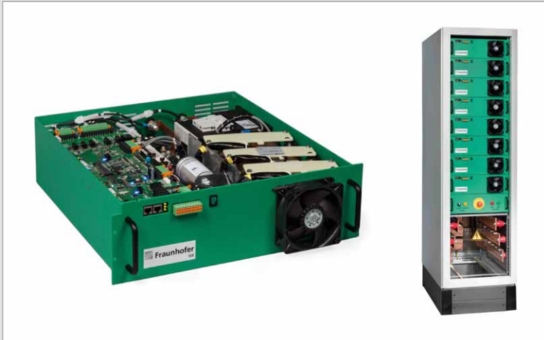
Figure 14: MV-HESS-inverter, single module and rack (Source: Fraunhofer Institute for Solar Energy Systems ISE).
